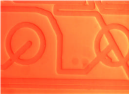
Figure 10: Microchannels etched in LCP material patterned with the SF-100 and etched with KOH
