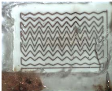
Figure 4: An optimized resistor with PDMS-walled-reservoir used for thermo-pneumatic actuation made in LCP with Cu/Zn conductors.
