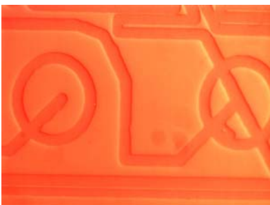
Figure 5: Microchannels etched in LCP dielectric polymer.
