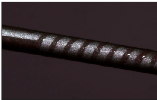
Helical Pattern of Positive Photoresist on a 1 mm Diameter Stainless Steel Rod
