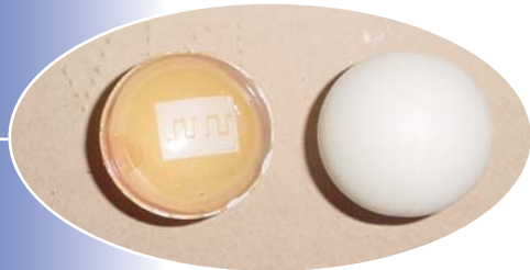
Photoresist Pattern on Internal Surface of Round Substrate. (Diameter=3 cm)
