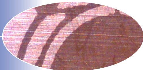
Detailed View of Diaphragm Section of Sensor (60X)
