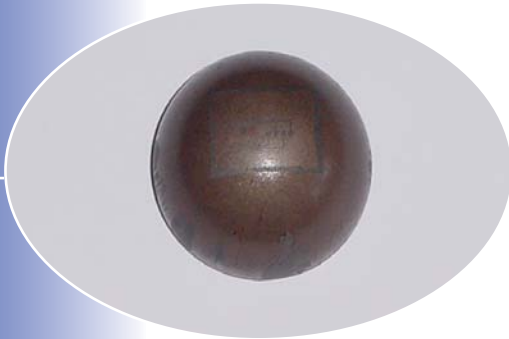
Photoresist Pattern on External Surface of Nickel Plated Substrate.
