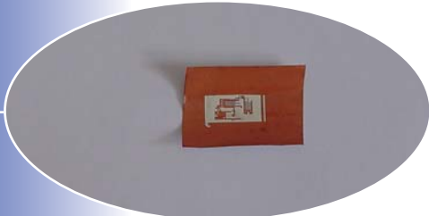
Thin Film Accelerometer (Device Dimensions 16 mm x 13 mm)
