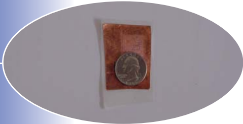
Photoresist Patterns on Copper Coated Mylar Substrate.
